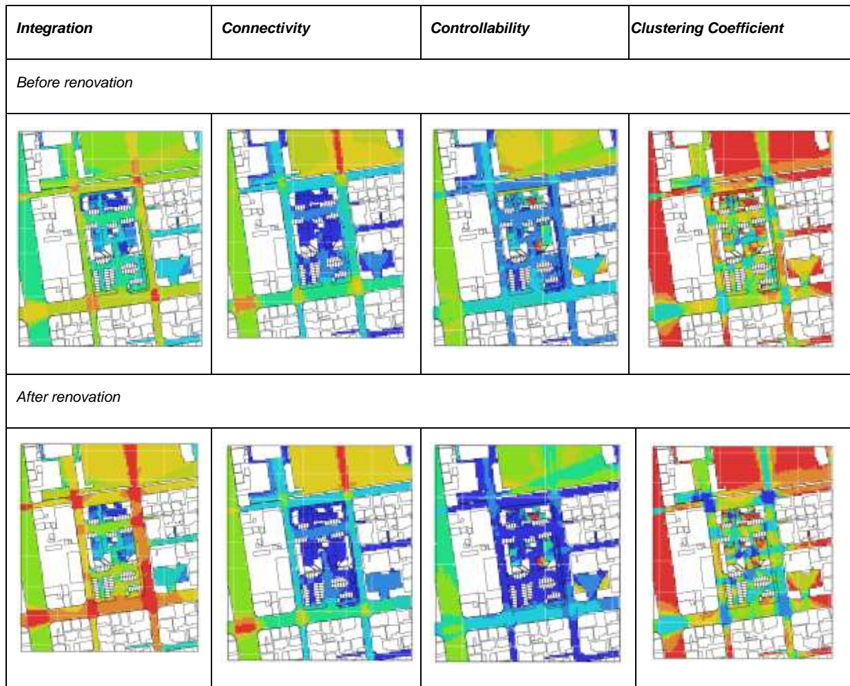
Figure 9. The Example of Visibility Graph Analysis Case 3. Removing inaccessible fences and walls
